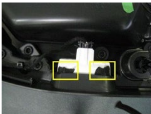
Figure 18. Fleece tape applied to light assembly.
