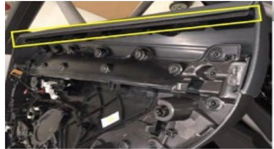
Figure 4. Fleece tape applied to mounting strip.
