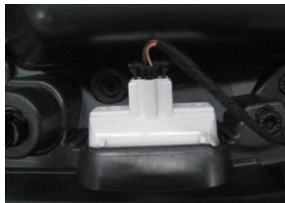
Figure 17. Wrapping light wire harness with fleece tape.
