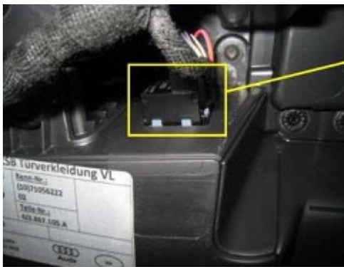
Figure 21. Apply fleece tape to pocket lighting.
