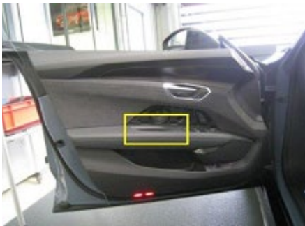
Figure 8. Isolate pull handle from armrest.
