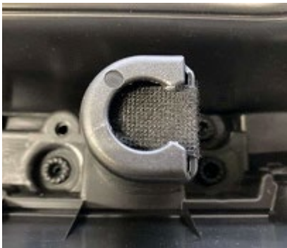
Figure 6. Door clip with fleece tape applied.
