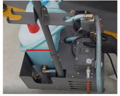
• For cleaning equipment, make sure to turn on the water pump first and then turn on the air. After turning on the air, visually check whether the air comes out from the end of the inlet of the equipment. When air does not come out, operate the air pressure valve to increase the pressure a little to check that air comes out and set it to 2 bar.
