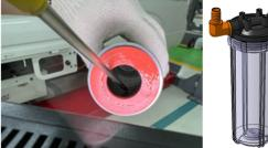
• Sludge can get stuck to the inner wall of the filter gaps, be sure to clean the filter evenly.
