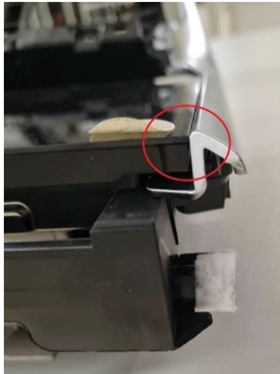
Figure 1. Hard contact between lower MMI display and center console insert/trim.
