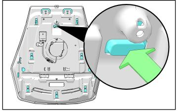
5. Locate the switch and heating element connectors on the bottom of the seat base.
