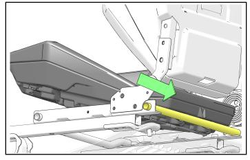
11. Press down on the seat base until it snaps into place over the base bar.
