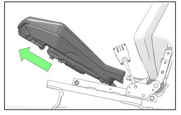
4. To remove, press the locking tab and slide the foam cushion forward to disengage the lower panel from the cushion.
