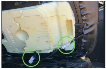
6. Locate the fan motor connection.
