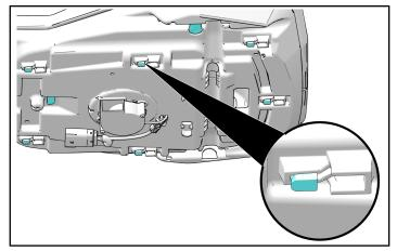
10. Install the seat base until the engagement recess is seated on the base bar.
