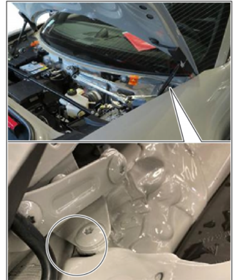
Seam sealing incomplete
