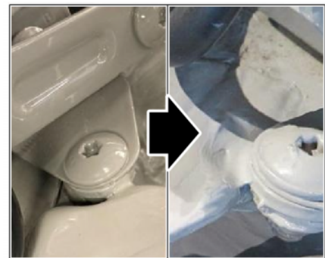
Applying sealing compound
