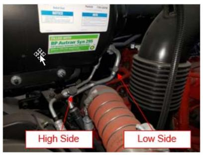
2. Recover the R-134 refrigerant from the vehicle's air conditioning system. *Refer to the R-134 Refrigerant Recovery, Recycle and Recharge manual of the machine being used.*
