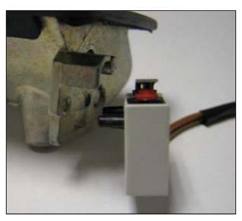
To install micro switch, align mounting tabs with handle alignment holes.
