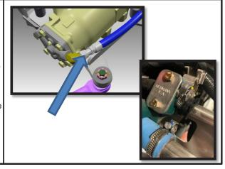
Step 5. Install new hose (N95797-02) with new clamp (N80726) on to the pump reservoir piping ensuring the hose is past the raised portion of the pipe. Place hose clamp 1mm from the end of the hose and Torque clamp to 3.25 ± 0.25 NM. or 27 to 31 lbs-in.
