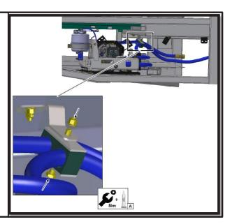
Step 8. Fill steering reservoir to max level mark located on the reservoir with CASTROL TRANSYND SYTH ATF N30283
