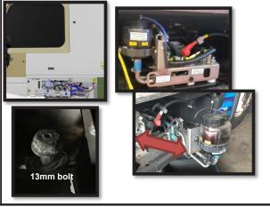
Step 3. Remove the four-hose clamp bracket hardware and bolts from the damage hose.
