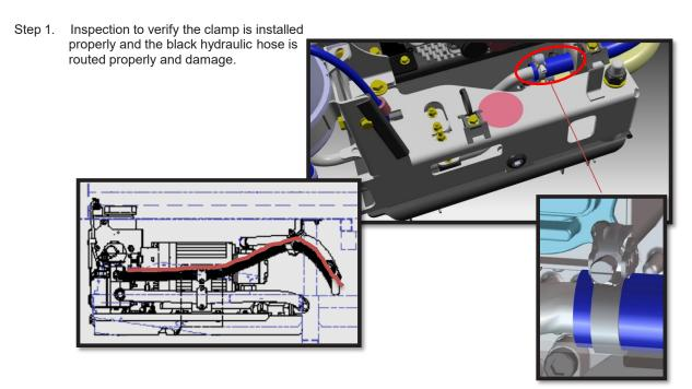
If the clamp is crushing the hose (restricting the flow), the hose and clamp needs to be replaced.
