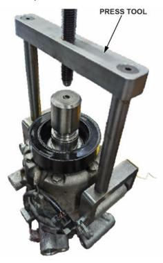
37. Tighten the press by rotating the handle clockwise until it reaches the adapter tool. Slowly and carefully continue to rotate the handle clockwise until the seal is pressed down roughly **10 mm** below the bore.
