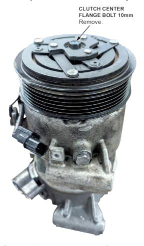
11. If the clutch has not been removed from a previous step, remove the clutch while being careful not to drop/lose any shims (usually 1–2).
