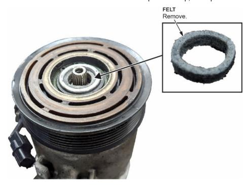
13. Remove the pulley C-ring.
