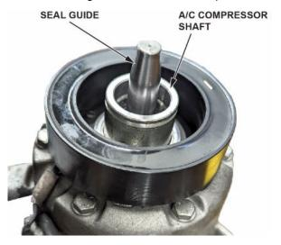
32. Insert the new seal onto the seal guide tool.
