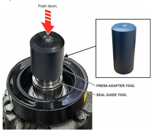
35. Insert the seal C-ring with the teeth's rounded side pointing down into the bore.
