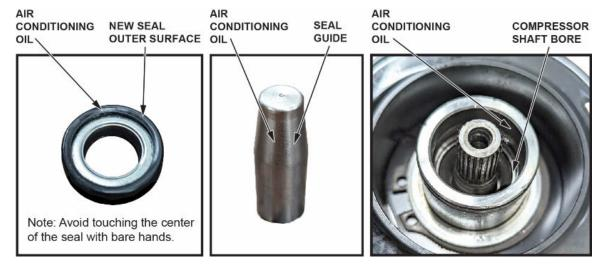
31. Insert the seal guide tool onto A/C compressor shaft.
