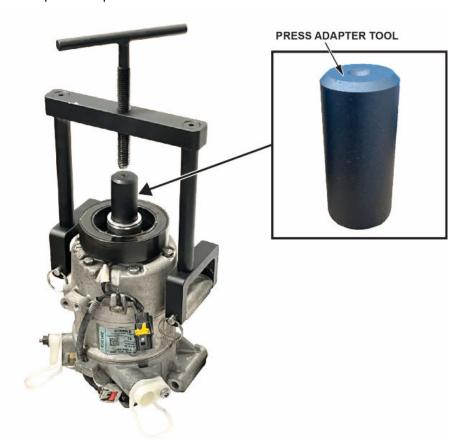
20. Add grease to the press adapter button and press threads.
