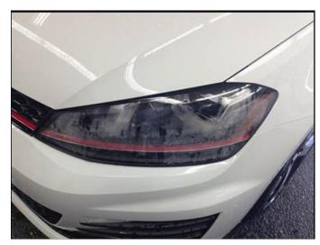
Exterior light assemblies (headlights, taillights, fog lights, turn signals) are vented and may collect moisture on their inner surfaces, depending on humidity and climatic conditions. The unfavorable condensation built up (Figure 1) visible to the customer is more common with modern exterior lights because of clear glass optics, however this condition will not have an impact on the functionality or durability of the component.
