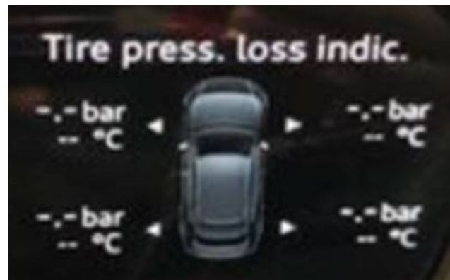
Figure 1. Tire pressure and temperature not available in the cluster.
