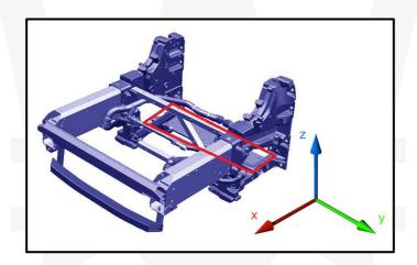
In case of noise like that shown in the attached videos, it is recommended to lift the car on the hoist and apply commercially available long-life spray grease (such as Würth HHS 2000) in the points shown below. The grease must be applied evenly, at the riveted joints, along the mating surface (see yellow rectangles).
