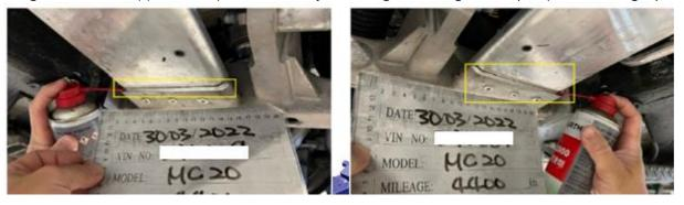
Once the operation is finished, clean off any excess grease and carry out a functional test.
