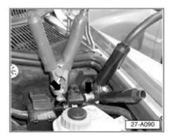
When using remote location terminals -arrows-, located in engine compartment, always reduce DIN rating on MCR340V, INC-940, VAS6161 and GRX3000 testers.
