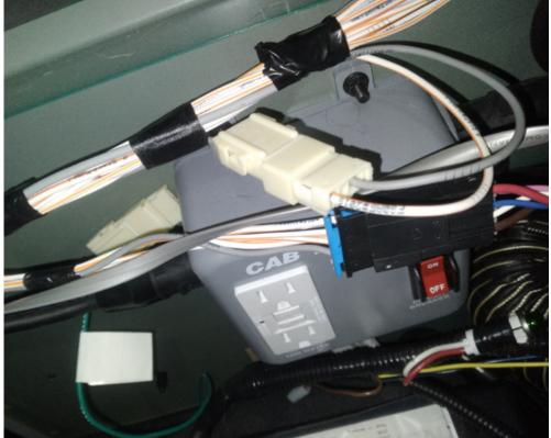
This connector should not be connected together. These connectors are not used.
