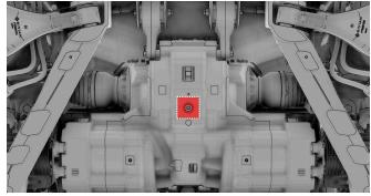
3. Drain the rear drive unit fluid into a measured container (refer to service manual procedure 421030024).
