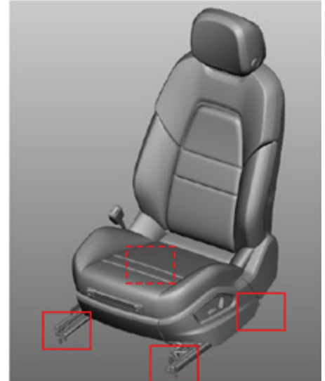
Figure 2: Seat mounting bolt locations
