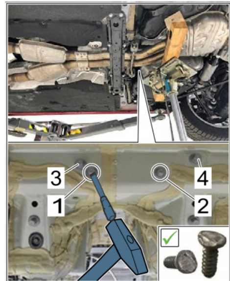
Removing fastening bolts
