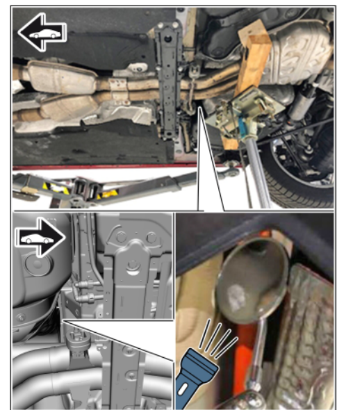
Checking floor pan
