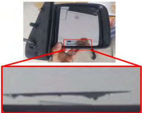
Erosion into the door mirror
