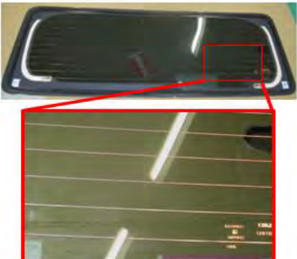
Discoloration of tailgate glass
