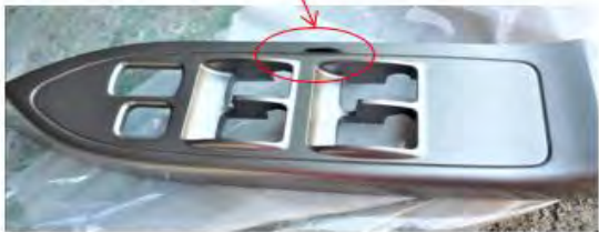
Peeling paint on the door switch panel
