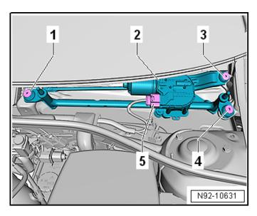
Reinstall wiper linkage in the reverse order of removal according to the ELSA Repair Manual.
