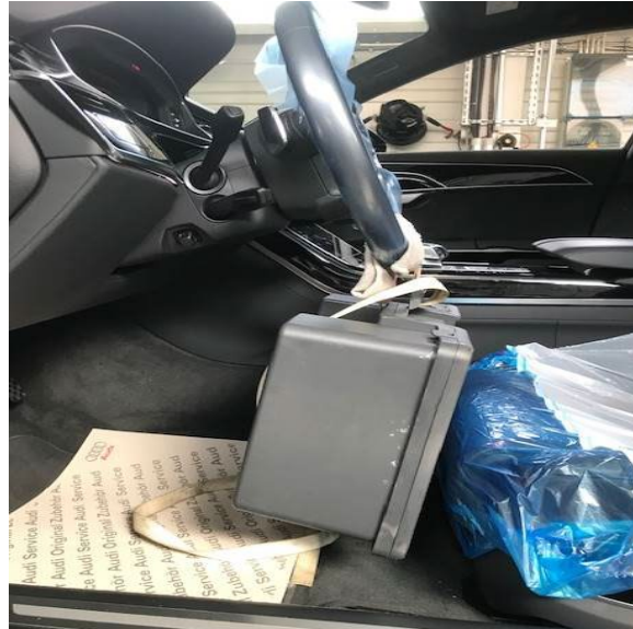
Figure 2. Weight necessary for steering adjustment.
