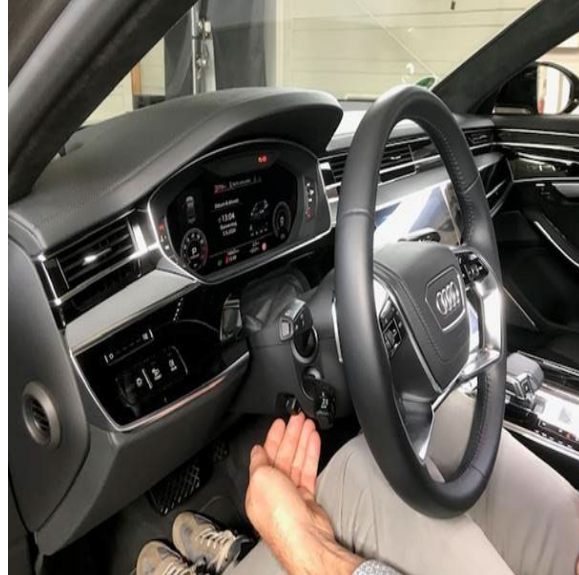
Figure 1. 40 kg force pushing steering wheel upward.
