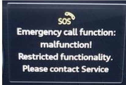
Figure 1. Emergency call malfunction warning.
