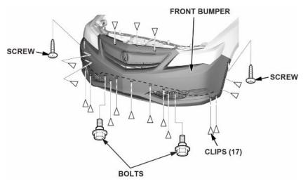
2. Pull out the front bumper at the wheel arch area to release it from the hooks on the side spacer.
