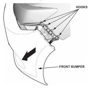
3. With the help of an assistant, while pulling the front bumper away from the side spacer, release the bumper from the hooks on the upper beam.
