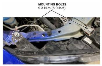
11. With help of an assistant, place the bumper back on the vehicle and install all required bolts and clips.
