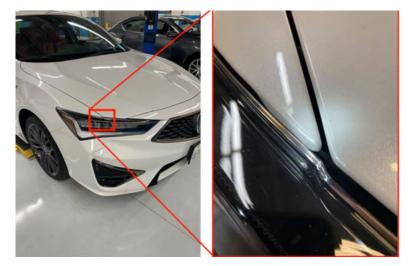
3. There should be clearance between the headlight and the fender as shown below.
