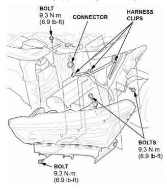
7. Remove corner upper beam from bottom of headlight.
