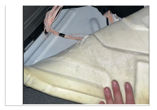
• Disconnect the two harnesses and verify that the no-start condition has cleared.
