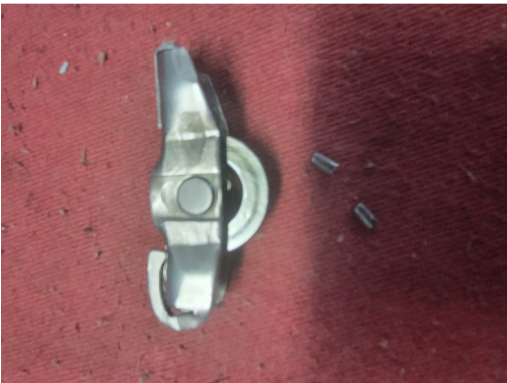
(Picture below shows example of excessive axle pin wear)
