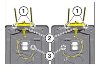
**YES** = Head restraint mechanism is faulty. Determine root cause of Bowden cable not moving (see steps below). If the cable is moving fully but the headrest is not folding, then replace the folding module of the head restraint (#2 in picture).
