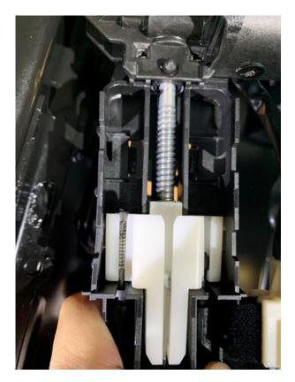
**NO** (Latch is closed) = Check if the drivetrain for backrest release adjustment is broken?
