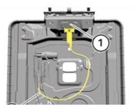
**NO** = Check if the Bowden cable is correctly mounted and properly routed.
