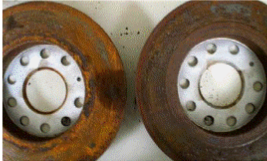
Figure 1: Example of excessively rusted disc brakes. Figure 2: Example of rusted disc brake surface.
