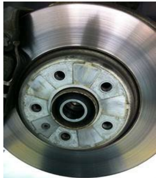
Figure 3. Brake disc with heat marks.
