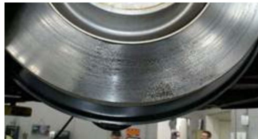
Figure 5. Pad marks on the brake disc.
