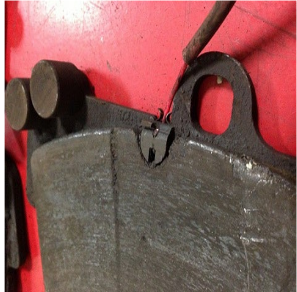
Figure 7. Worn brake pad.
