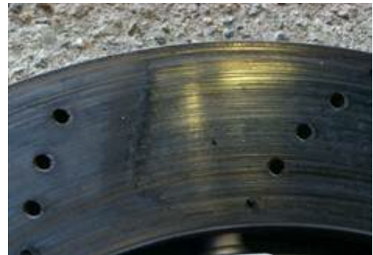
Figure 2. Deposits on the brake disc.
