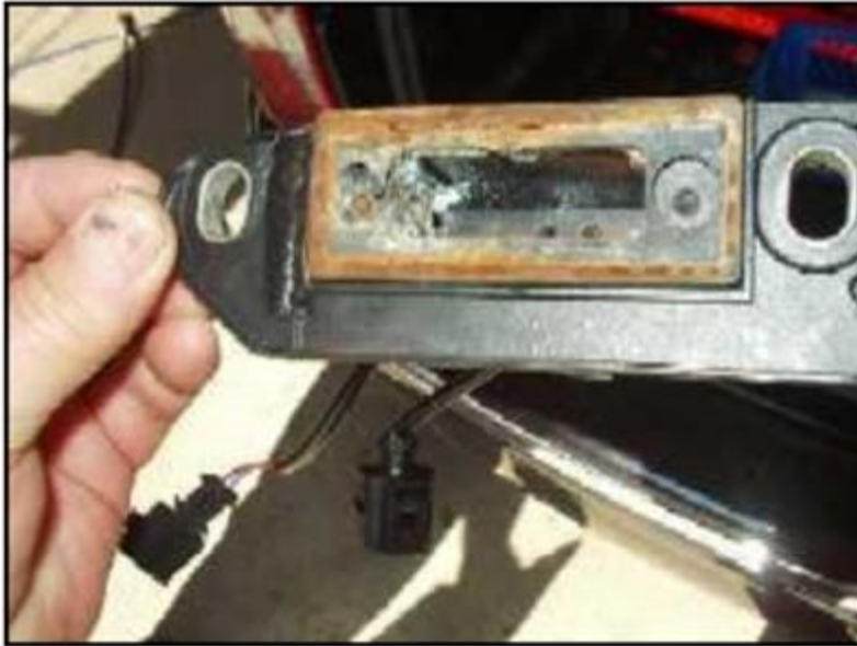
Figure 2 – Corrosion around License Plate Light
