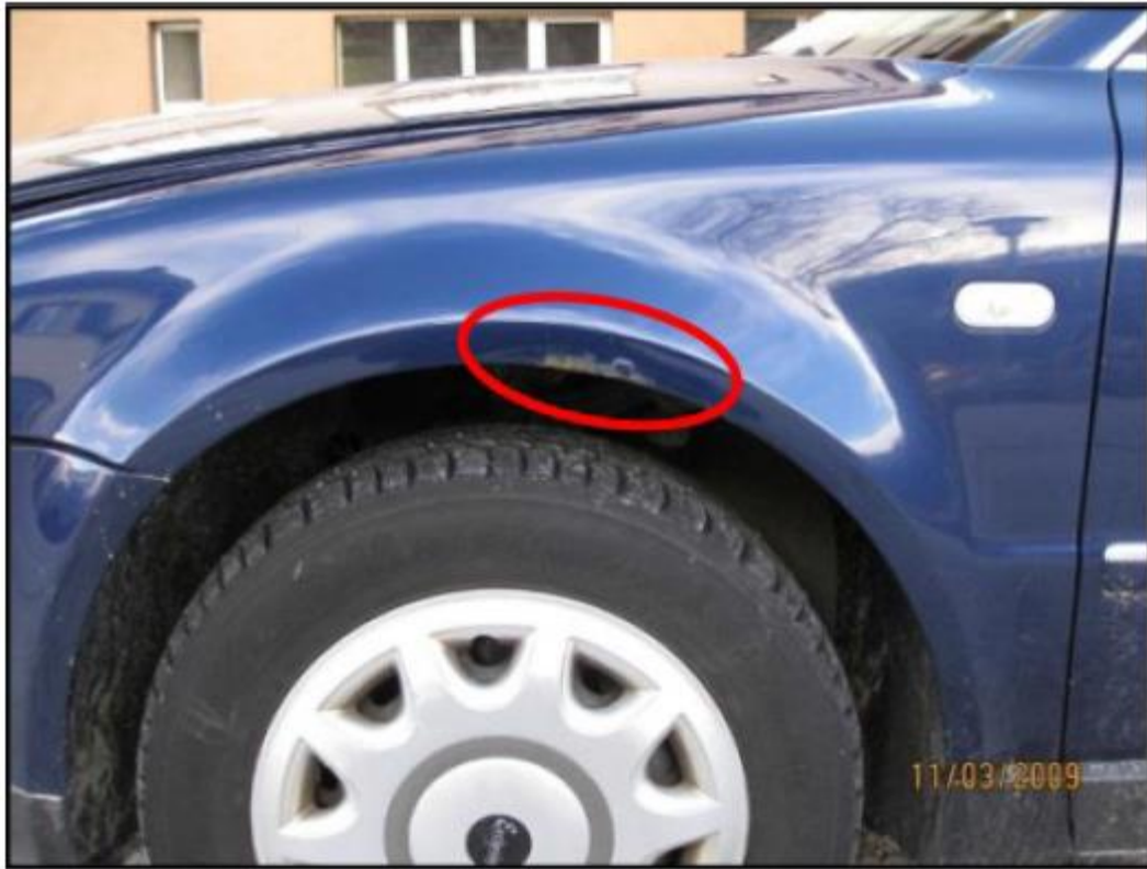
Figure 1 (corrosion on left wheel arch)
