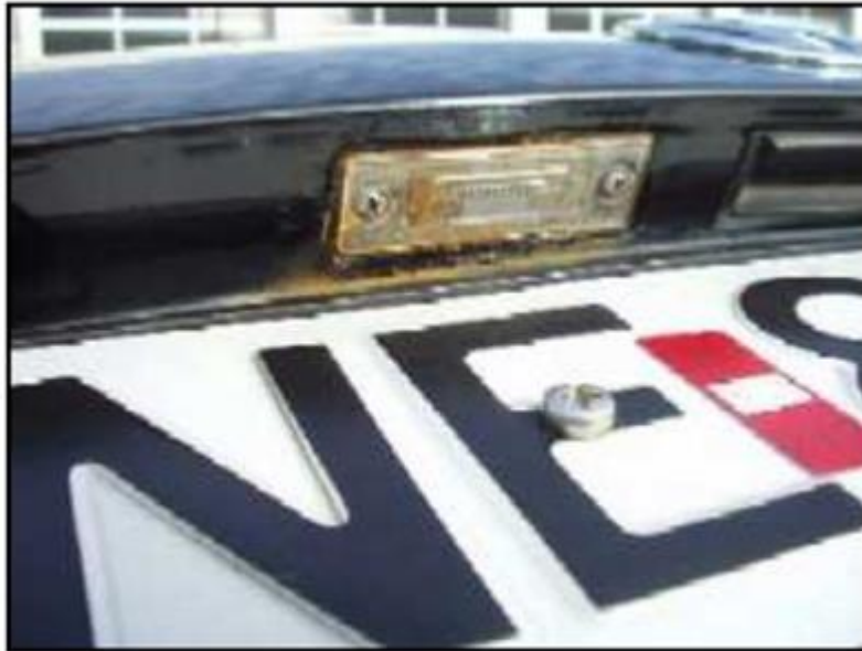
Figure 1 – Corrosion around License Plate Light
