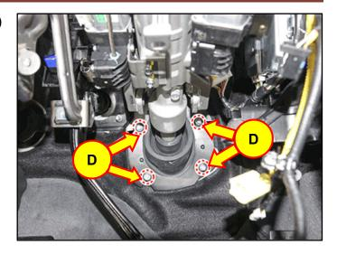
4. Clean the universal joint shaft with a cloth to wipe off foreign substances and grease.
