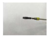
Remove terminal completely from the VCI connector and inspect the locking tab. (see picture below) If the tabs are ok reinsert the terminal in the VCI connector and pull on wire with steady force to ensure positive lock of the terminal. Push the yellow lock tab back down when completed.
