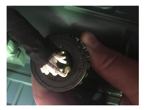
Examples of terminals not properly locked in the VCI connectors causing electrical faults. See pictures below
