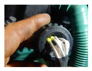
**NOTE:** If terminal will **NOT** properly lock in the VCI connector, the external engine harness will **NEED** to be replaced.
