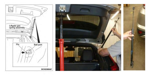
3. Install the new liftgate gas spring assembly. Connect the liftgate gas spring and the ball joint in the direction of the arrow.
