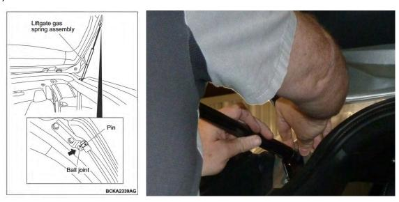
4. Push the pin to lock the liftgate gas spring and ball joint.
