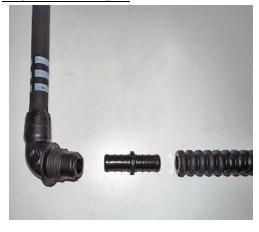
Install a rigid plastic tube into the panoramic sunroof drain hose.
