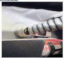
The panoramic sunroof drain hose has been over-sprayed with either paint and/or clear coat at the plant, causing the hose to tear at the top due to vibrations/body flex in the vehicle.
