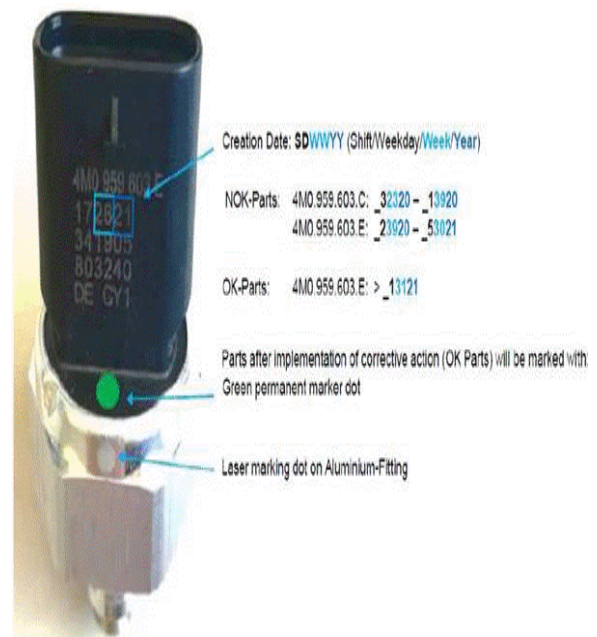
Figure 1. Pressure and temperature sensor markings and build date.
