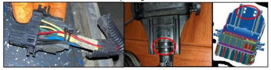
Install backshell onto connector Connect two pieces of backshell together onto cable
