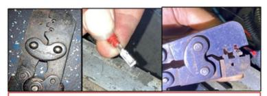
Terminal SLK 2.8 16-14AWG Kostal 22124492070 Install seal onto wire. Red seal (gasket) Kostal 10800444523 Crimp terminal onto wire. Use DELPHI GM12014254 Crimping tool
