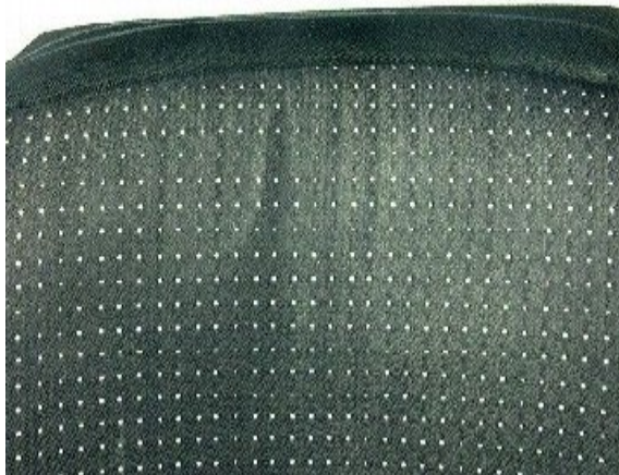
Figure 15. Lightening/greying of surface
