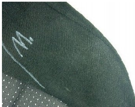
Figure 16. Lightening/greying of surface
