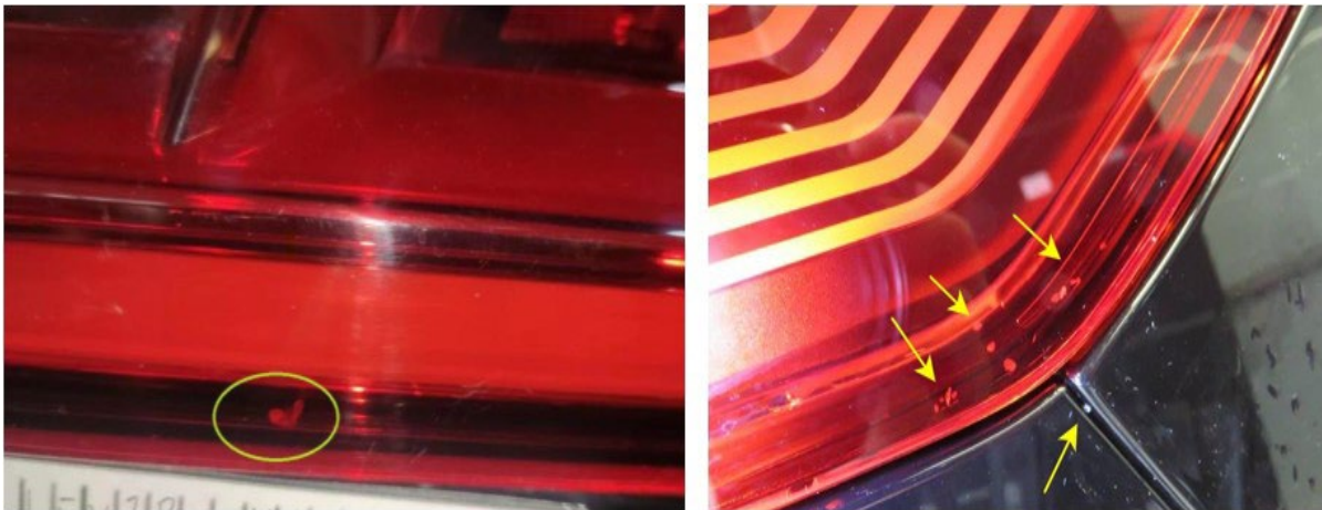
Figure 1: View of foreign objects (e.g. insects) inside of the tail light.
