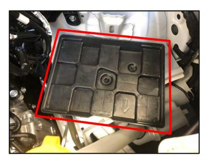
**STEP 4:** Install the original battery cover to the new replacement battery. Confirm the bottom of the cover is aligned flush with the bottom of the battery.
