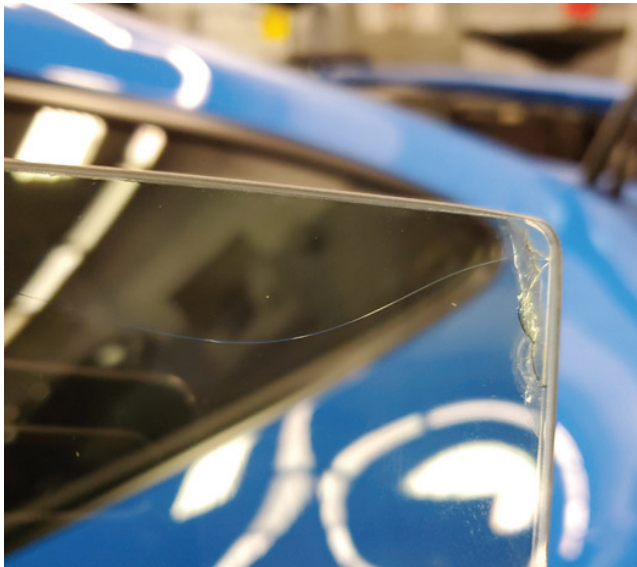
Figure 1 - Door glass: cracks in the top corner
