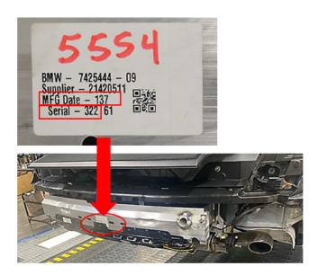
2. Check the production date and serial number on the rear bumper support label.
