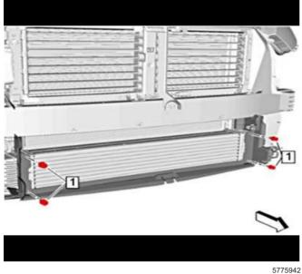
5. Remove and discard the 4 Lower Air Baffle push-in retainers (1), as shown in the picture above.
