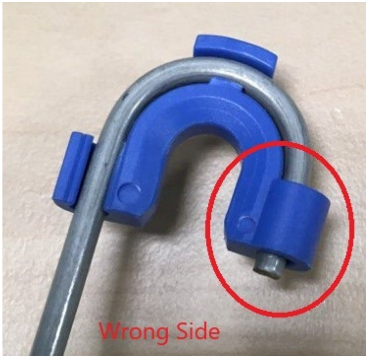
Figure 1. Spring clip installed incorrectly . Closed loop on short side of tension spring.
