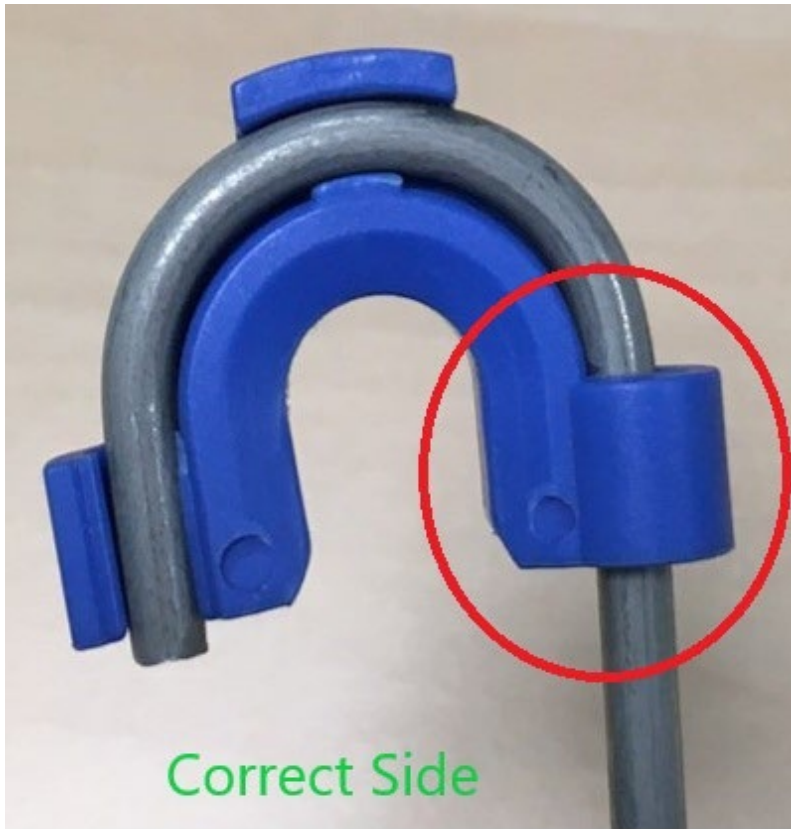
Figure 2. Spring clip installed correctly . Closed loop on long side of tension spring.
