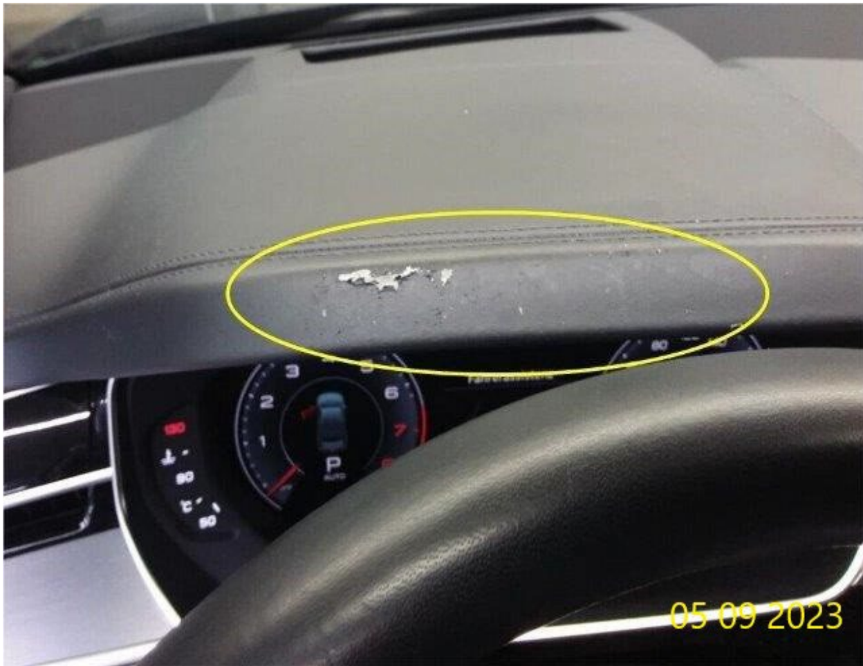
Figure 10. Leather detachment due to the use of harsh cleaning agents.
