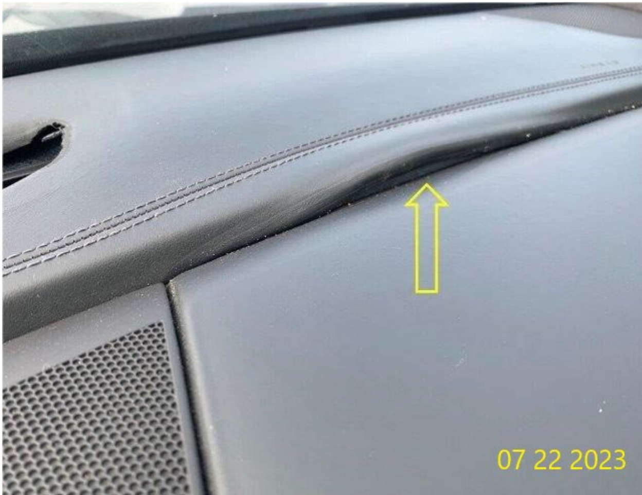
Figure 4. Delamination at the bend / radius.
