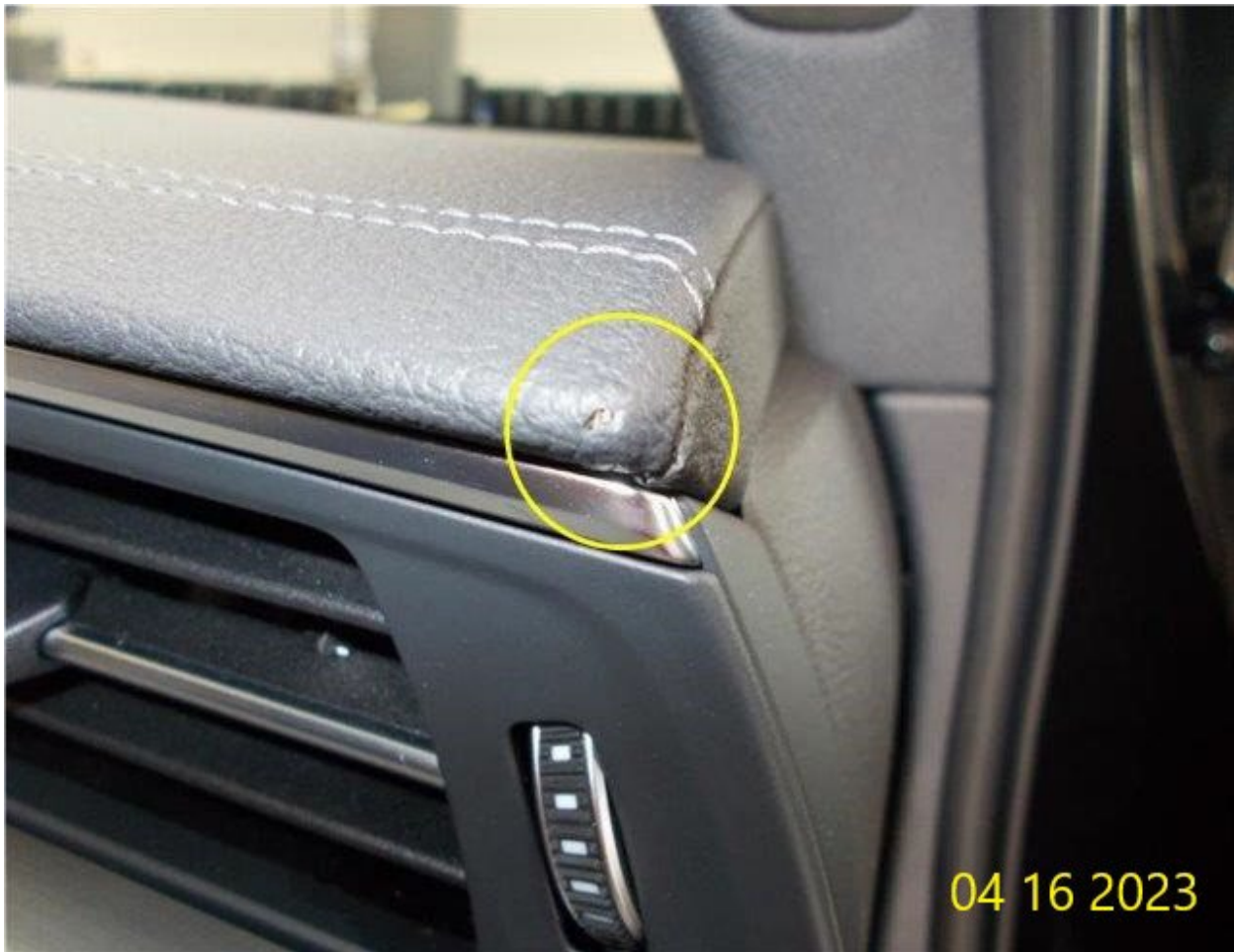
Figure 9. Leather damaged by mechanical force.
