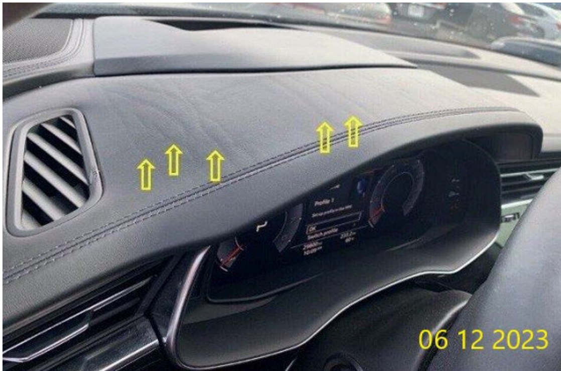
Figure 6. Wrinkles due to shrinkage.
