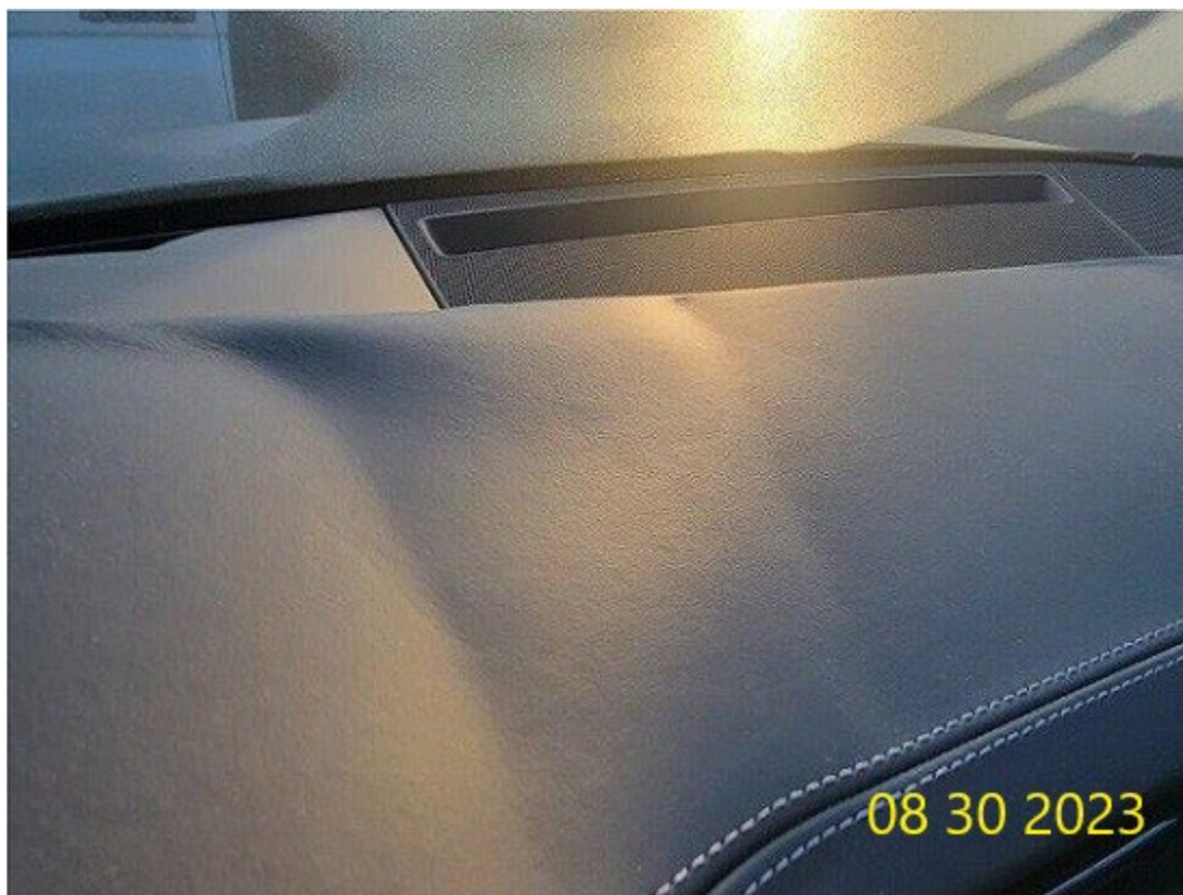
Figure 2. Massive, large-scale delamination.
