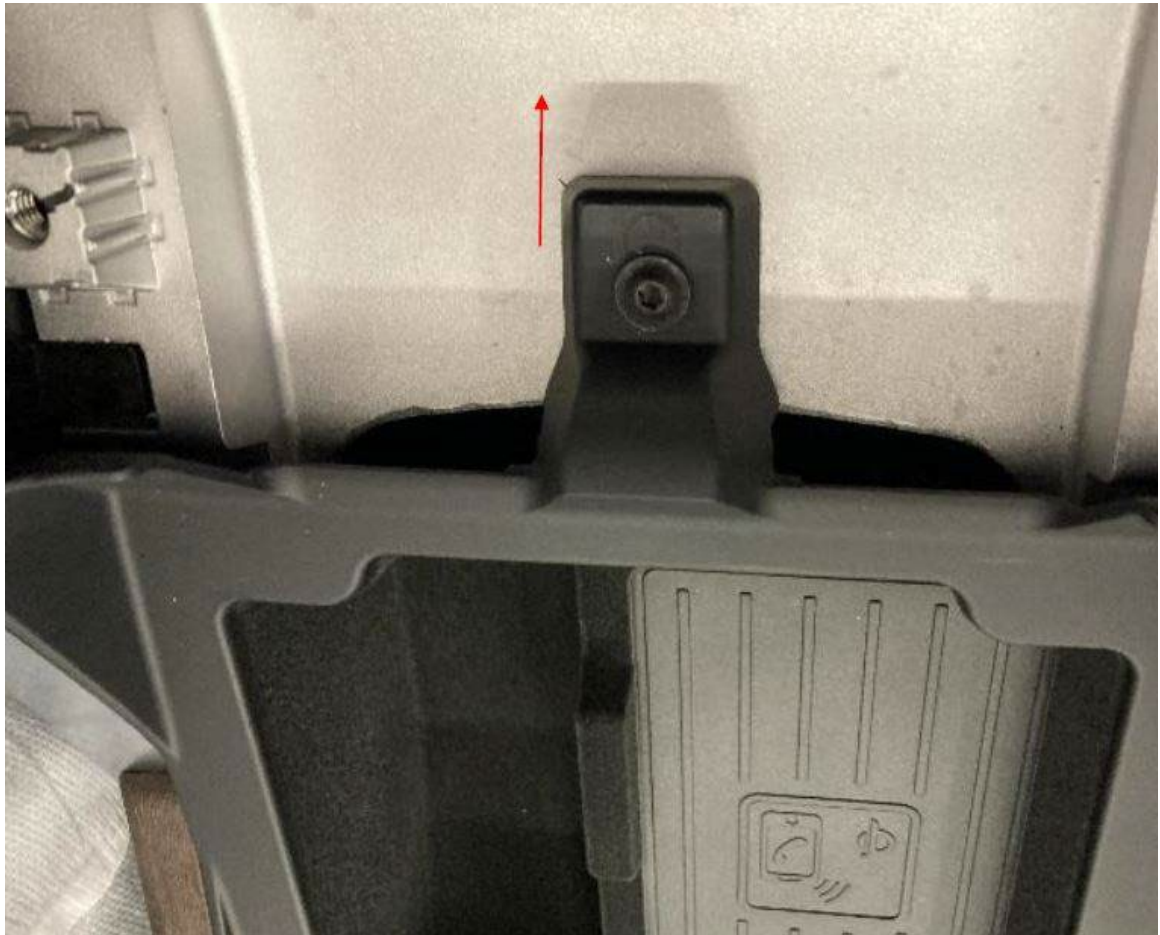
Figure 2. Moving the center console upper section towards the rear of the vehicle
