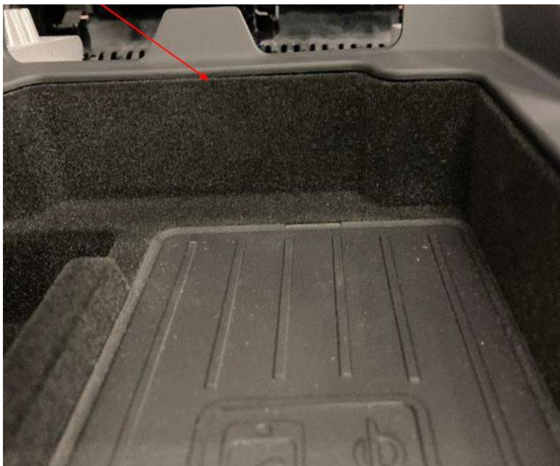
Figure 3. Center console upper section to storage bin gap, even and approx.0.5 mm wide.
