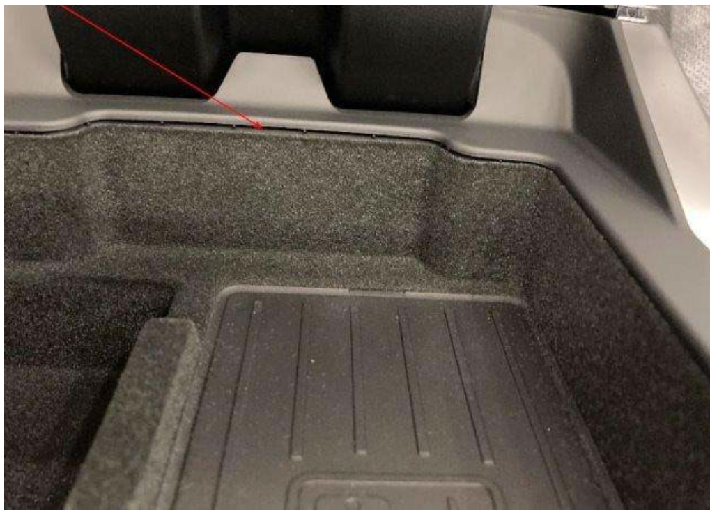
Figure 1. Check the gap between the center console upper section and the storage bin.
