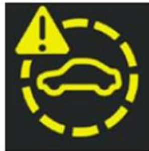
Figure 2. Symbol for “Audi pre sense not available at the moment” (MY2021 and on).
