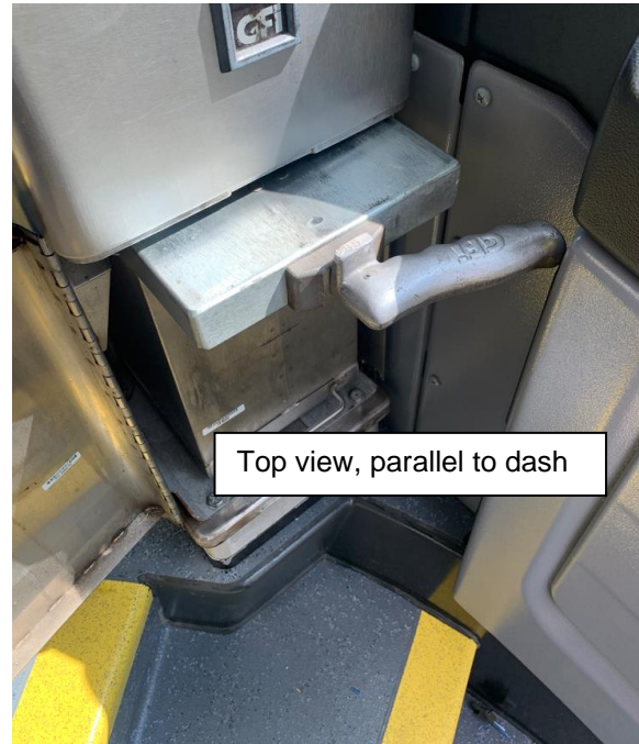
FIGURE 2: SHOWN INTERFERENCE ISSUE WITH THE DASH PANEL
