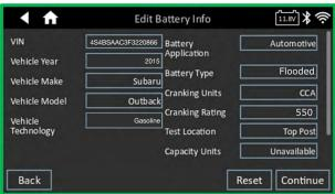
Once the battery information is confirmed and accurately entered, select "Continue" to proceed with the battery testing.
