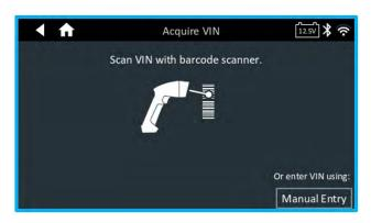
**NOTE:** In a case where the scanner option is unavailable the VIN can be entered by using the manual entry function.
