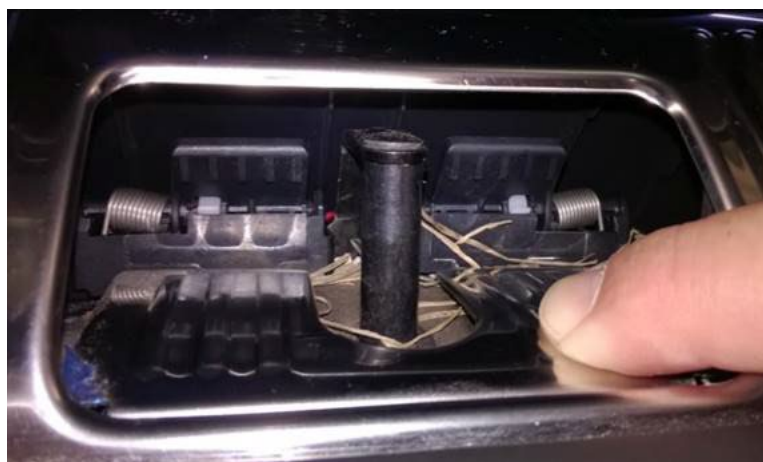
Figure 2: Dirt and debris interfering with the operation of the rear lid sensor.
