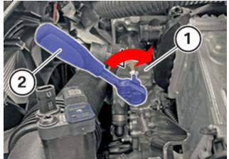
Cylinder 1 intermediate lever may interfere when trying to install the intake camshaft timing tools.
