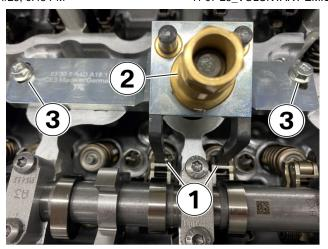
Special tool 83 30 5 A4D A18 must aligned properly with the rollers (1).
