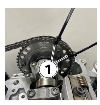
4. After the cylinder head cover is removed and before removing the exhaust camshaft place 2 wire ties (1) on the intake VANOS gear to hold the timing chain in place.
