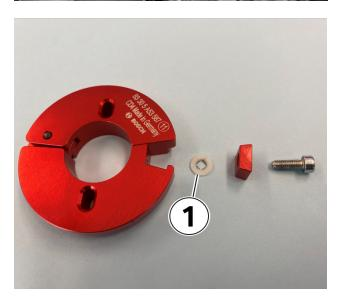
Tool 83 30 5 A53 587 may bind when removing it from both of the VANOS adjusters, the plastic washer (1) may be binding the tool and will not allow it to collapse when the screw is loosened.
