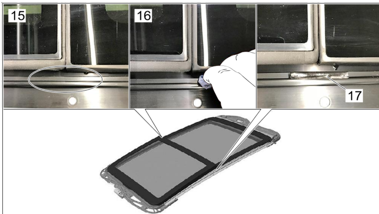
Butyl lock centered on roof assembly frame
