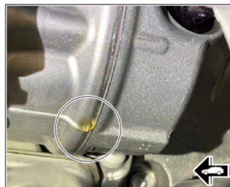
Drop formation on air-conditioning compressor
